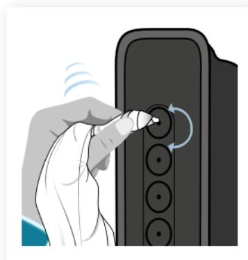
> Clean the needles of the device by forming a point with a dry cloth and turn it in each of the ionic optics. Repeat the operation at least twice a year.
