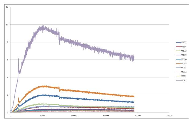
The artefacts observed at t = 1200 and t = 8000s correspond to the removal of a low-pressure electrostatic impinger ELPI + in order to determine the size of the particulate aerosol observed (Cf following paragraph).
