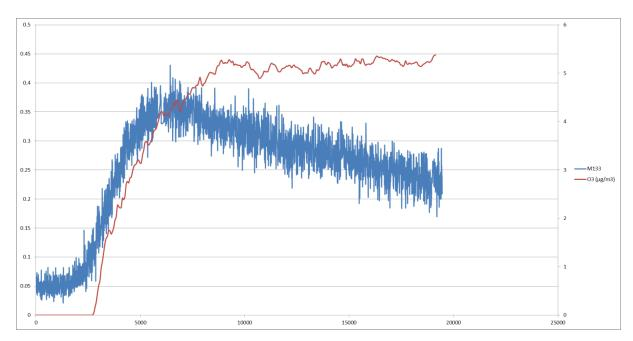
During the evaporation phase of the terpenes, the ozone concentration measured in the caisson increases from 0 to  $5.5 \,\mu g$  / m3 and stabilizes at t = 9180s.
