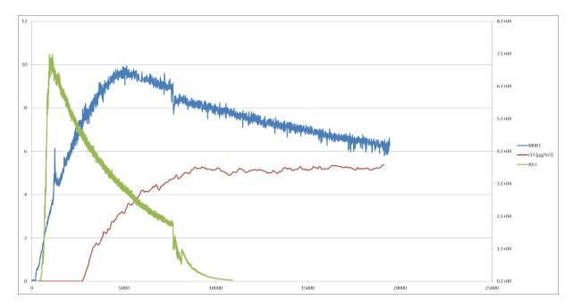
This aerosol, measured with ELPI, has a size between 40 and 60nm at the maximum particle concentration (t = 1050) and then forms droplets of greater size (100-300nm) by coalescence phenomena thus explaining the decrease of the concentration in number observed. Activation of TIP9 at t = 7678s causes a sharp rupture in the observed natural particle decay, thus confirming its action on suspended particles.
